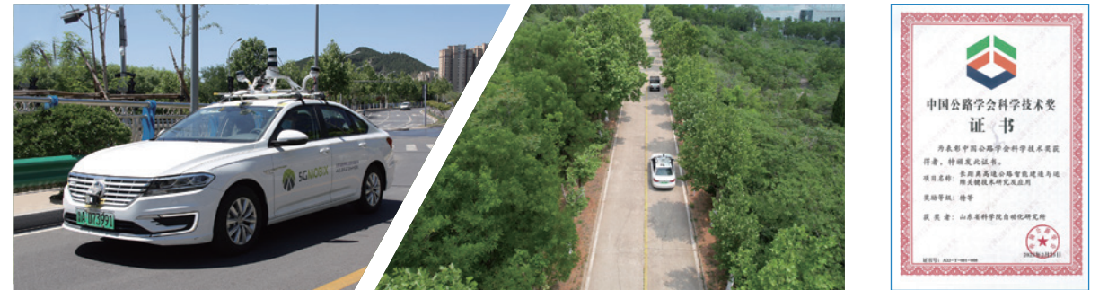
5G+自动驾驶智能车辆平台(L4等级自动驾驶功能) 5G+ autonomous driving intelligent vehicle platform (level 4 autonomous driving functionality)
